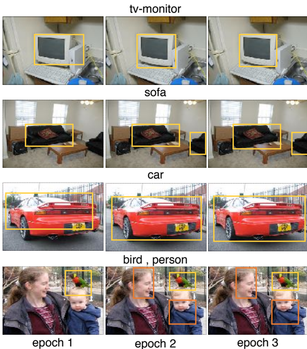
Figure 7: Examples of our generated box-level annotations. The yellow and orange boxes are generated by our dual-network approach and used as annotations for the next round training. Each triplet indicates the boxes generated in the same image from 1st epoch to the 3rd epoch.
