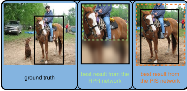
Figure 3: The two networks have different strengths which complement each other. The black box is the ground truth. The green box, generated by the Region Proposal Refinement (RPR) network, misses the lower part because it favors the bounding box which is occupied by the largest part of the object. The orange box, generated by the Positive Instance Selection (PIS) network focus on classification, and does not align well with the ground truth.
